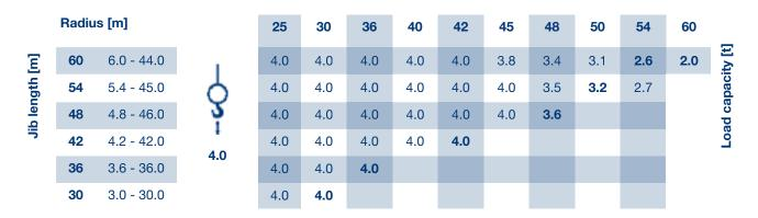
The loads relate to 45m hook travel. For longer hook travel distances, the loads are reduced by the additional weight of the hoist rope (with 1 fall rope = 1.3kg/m hook travel).
